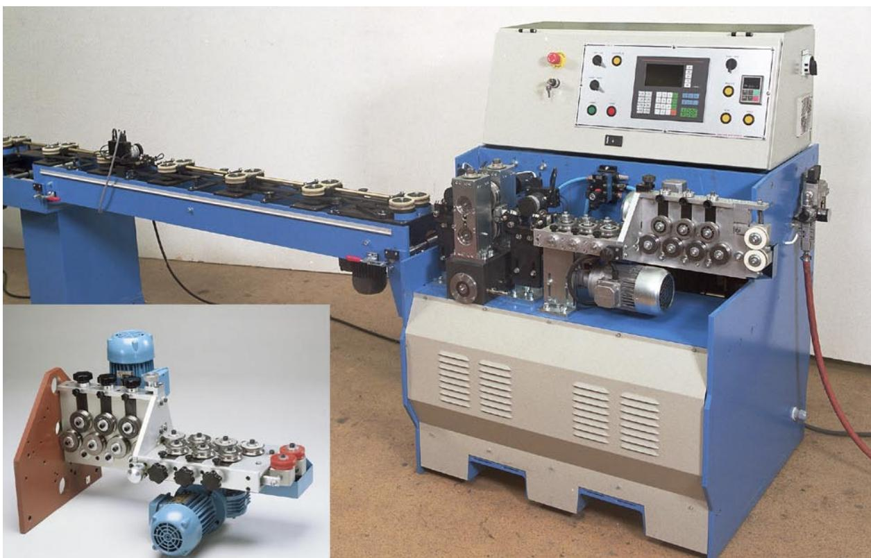
**GRANLUND length compensating machine, type KOL-R and straightening device, type KRO**
